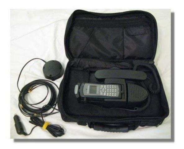
Hands free operation with speaker and microphone. Courtesy handset for privacy. Cig Adapter for power. (desktop cig socket power unit, 110v to 12 VDC available.) Puck like magnetic antenna comes with 15 foot cable. Extension to 50 feet available. Handsome cordura carry case standard. MSRP \$825 (requires phone).
